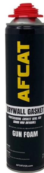
**C. Foam application:** Put on protective gloves. Shake the can well before use. Screw the can onto the applicator. Hold the can upside down and activate the foam by pressing the valve. Always handle the canister with the valve pointing downwards. Moisturizing the surfaces and the foam improves adhesion and shortens curing time. Vertical gaps should be filled with foam starting at the bottom and moving up. Do not fill the entire gap – the foam will increase in volume.
