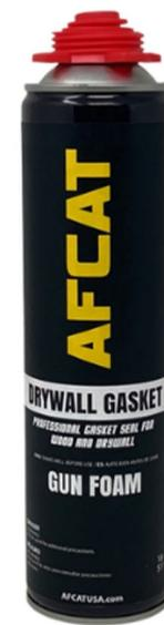
The foam maintains its usability within 12 months from manufacturing date, if it is stored in original packaging in vertical position (valve facing up) in a dry place in temperature +5°C to +30°C. Storage above +30 °C and below +5 °C shortens shelf life and properties of product will be affected. Storage of foam cans at temperature exceeding + 50°C or in vicinity of open flame is not allowed. Storage of the product in a position other than recommended may result in jamming the valve.
