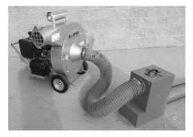
5. Attach hose or vacuum bag to the machine's outlet using a hose clamp.
