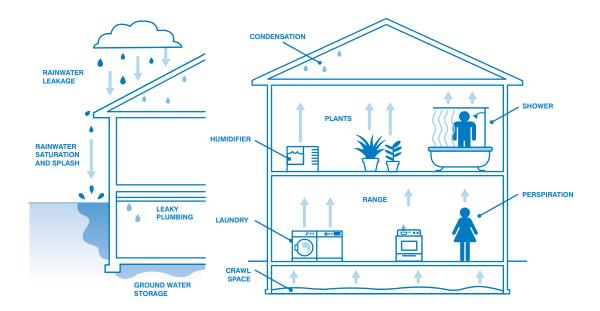
Moisture can enter the cavity from both indoor and outdoor sources. An average family of four can create two to three gallons of water vapor per day by cooking, bathing, washing dishes and doing laundry.
