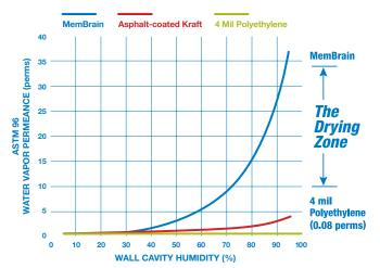
MemBrain can adapt from <1 to 35 perm to keep moisture out of the cavity in the winter while letting it escape when cavity humidity increases in the summer.
